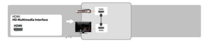
If the equipment has a DVI jack and not an HDMI jack, connect the DVI jack to the HDMI IN (with DVI-to-HDMI cable or adapter) jack and connect the audio jack to the PC AUDIO IN jacks.
